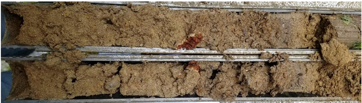
Plate 3 –Hf | Loose, silty sand | PG-2, S-1 @ 2½ – 4 feet.
