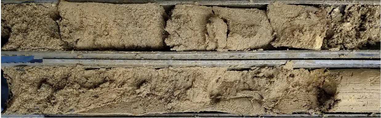
Plate 4 – Qylc | Medium dense SILT | PG-3, S-1 @ 5-6½ feet.
